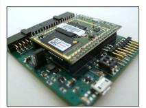
Custom kernel and modules; High-speed mixed signals PCB design, C firmware handling real-time sampling and DMA chaining, USB CDC and custom boot loader.
