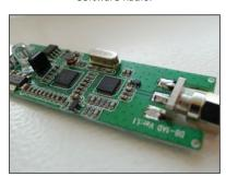
RTL chipset based software radio; GNURadio; audio signal processing; FLEX protocol & AMR decoding in MATLAB.
