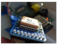
RaspberryPi; Custom Linux kernel with PPS (ATOM) support, NTP services; BASH scripts for headless operation; RRDTool based remote monitoring.
